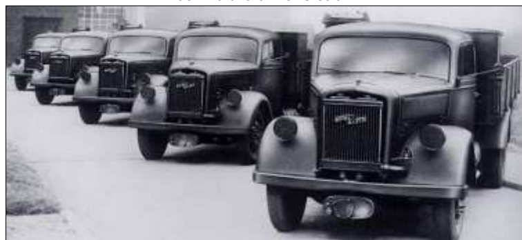
German trucks “Opel Blitz,” mass-produced during World War Two with producer-gas generators (behind the driver's cabin, passenger side).
